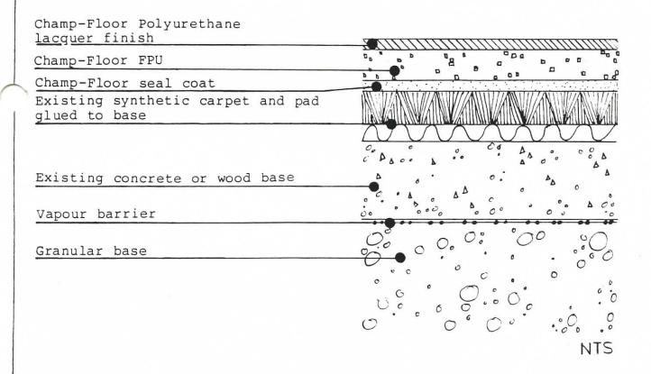
Note: It is important that the base - carpet - is cleaned to its original condition. The surface must be smooth and have a moisture content of less than 5%. Minor deviations in the level of the surface can be filled with the Champ-Floor material. Major deviations must be filled with the same material as the base.
